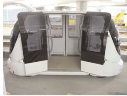
The tour included a close-up look at the battery-powered ATS vehicles.
